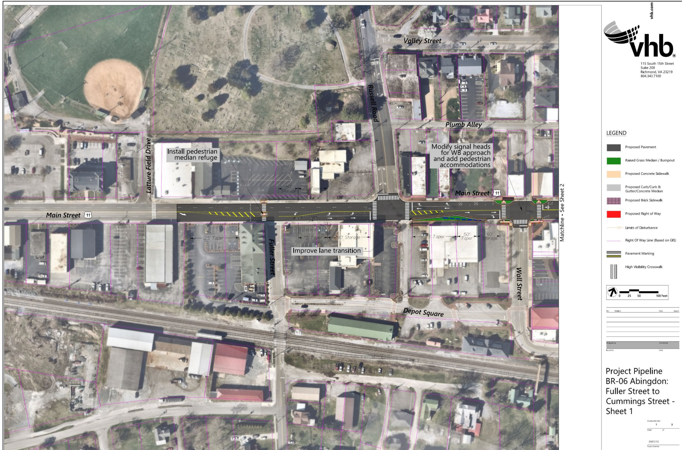
Figure 83: Fuller Street to Cummings Street Improvements - Sheet 1
