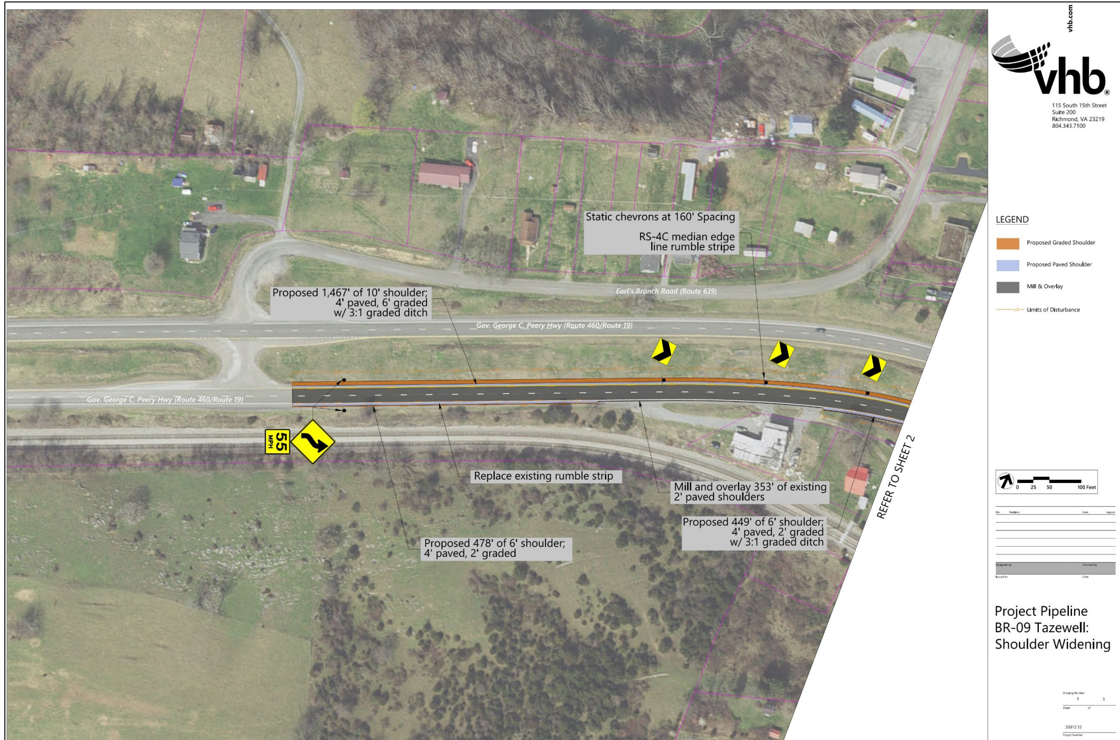
Figure 33: Shoulder Widening and Safety Improvements - Sheet 1
