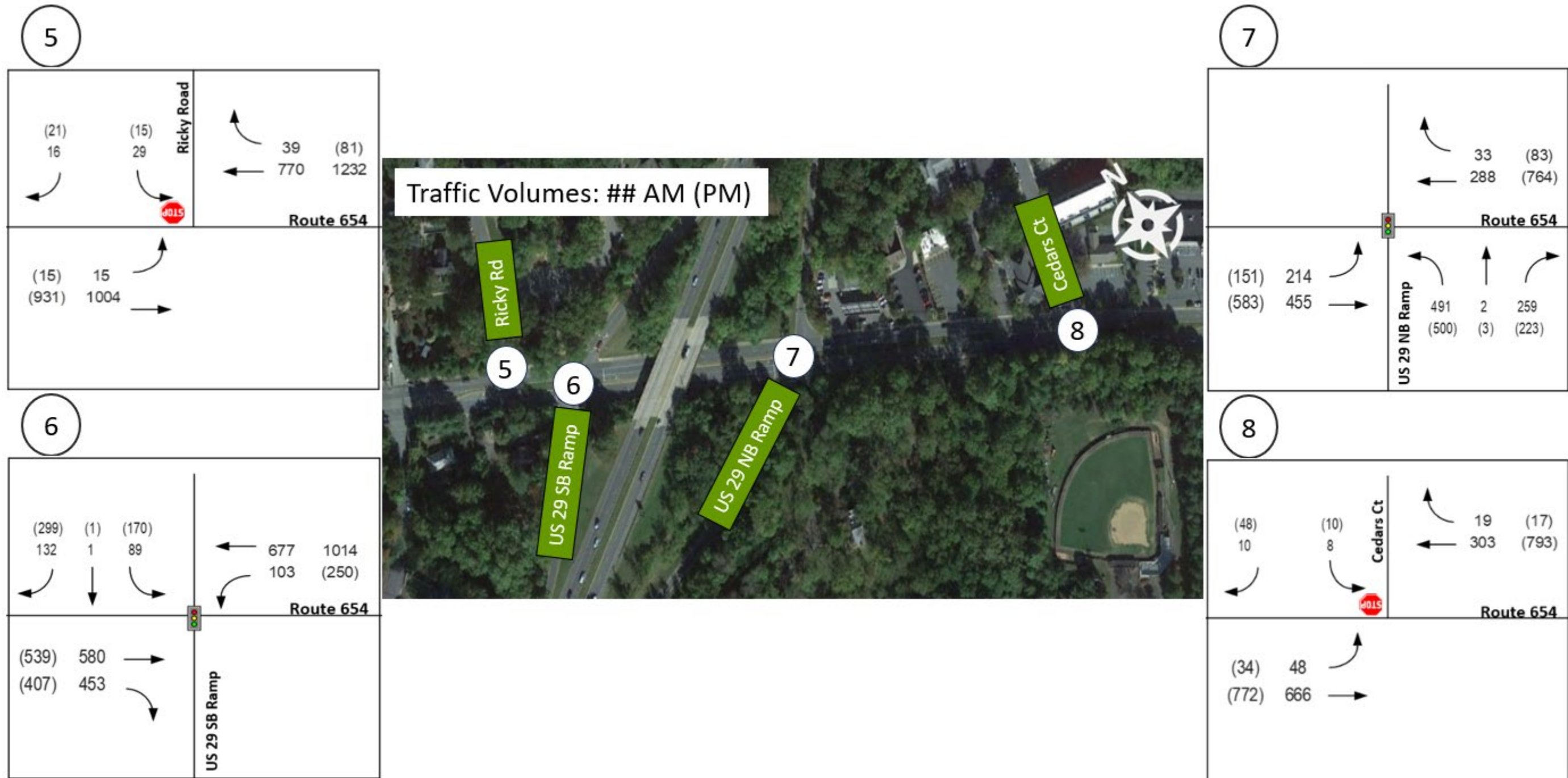
Figure 1-14. Barracks Road (Route 654) – Existing Conditions Peak Hour Volumes (2 of 3)
