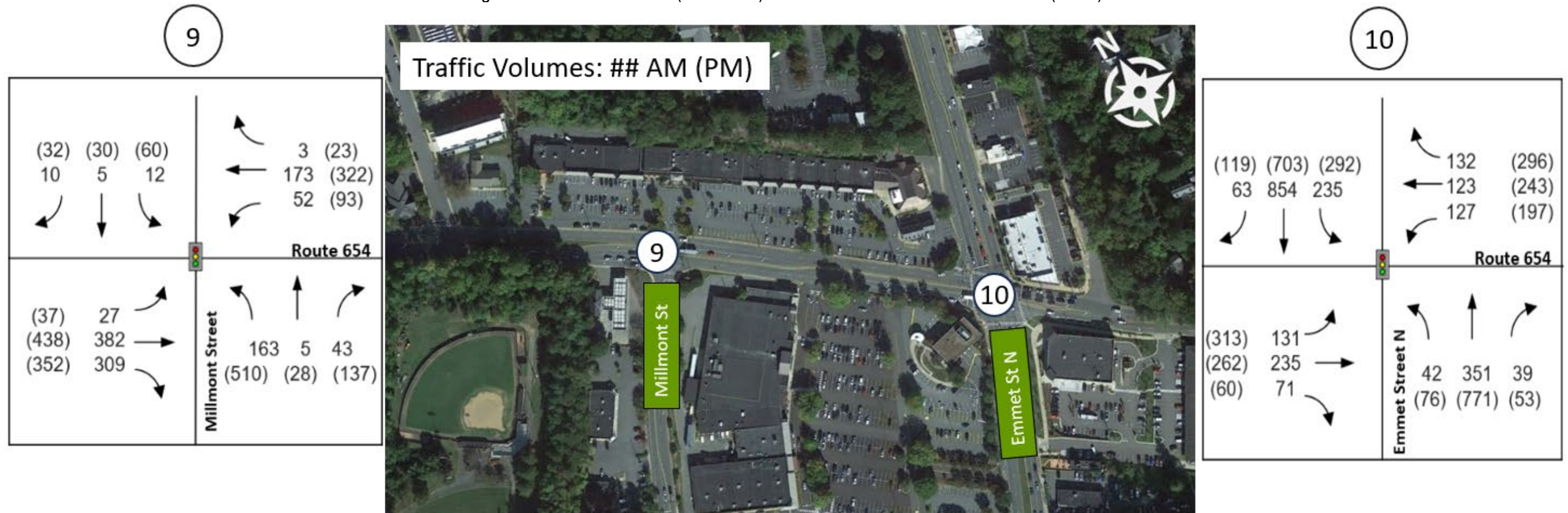
Figure 1-22. Barracks Road (Route 654) – 2035 Balanced Peak Hour Volumes (3 of 3)
