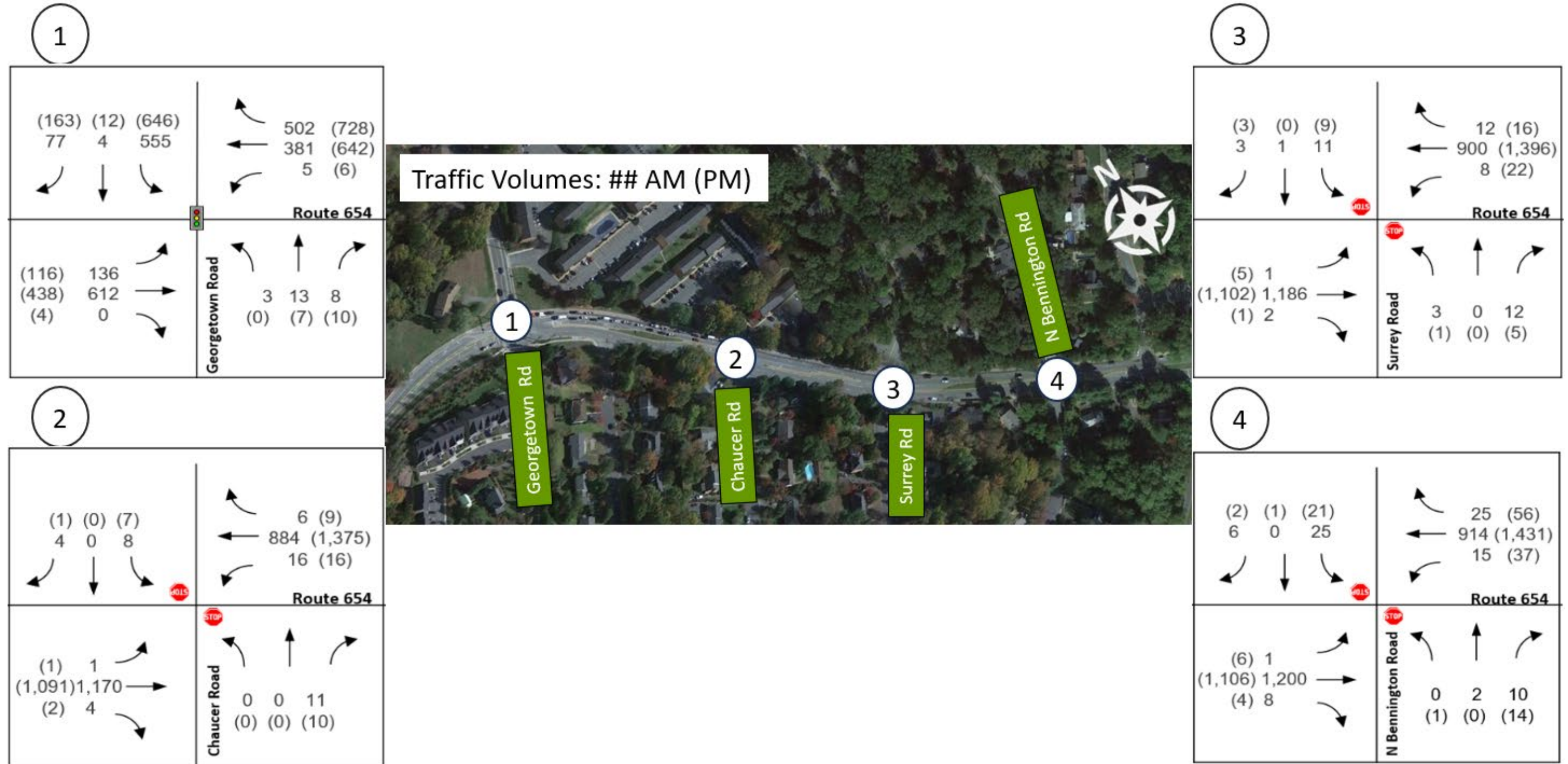
Figure 1-23. Barracks Road (Route 654) – 2045 Balanced Peak Hour Volumes (1 of 3)
