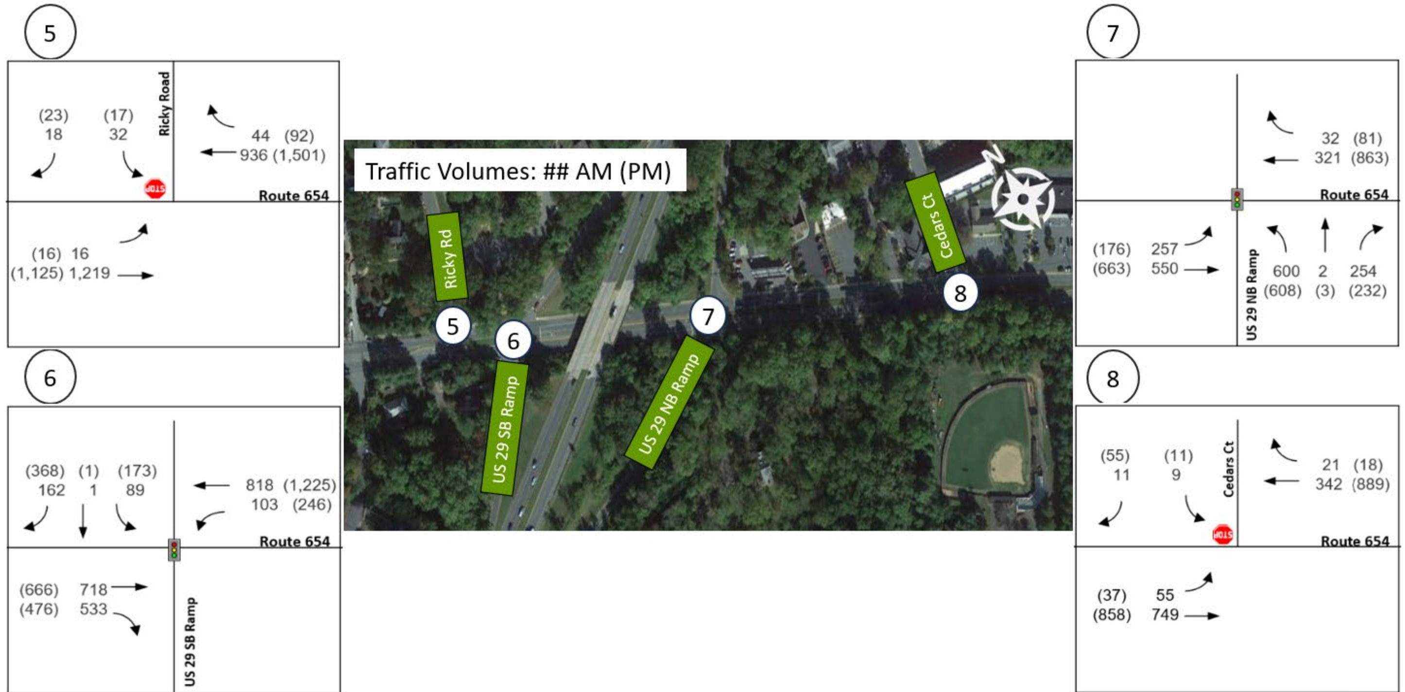
Figure 1-24. Barracks Road (Route 654) – 2045 Balanced Peak Hour Volumes (2 of 3)
