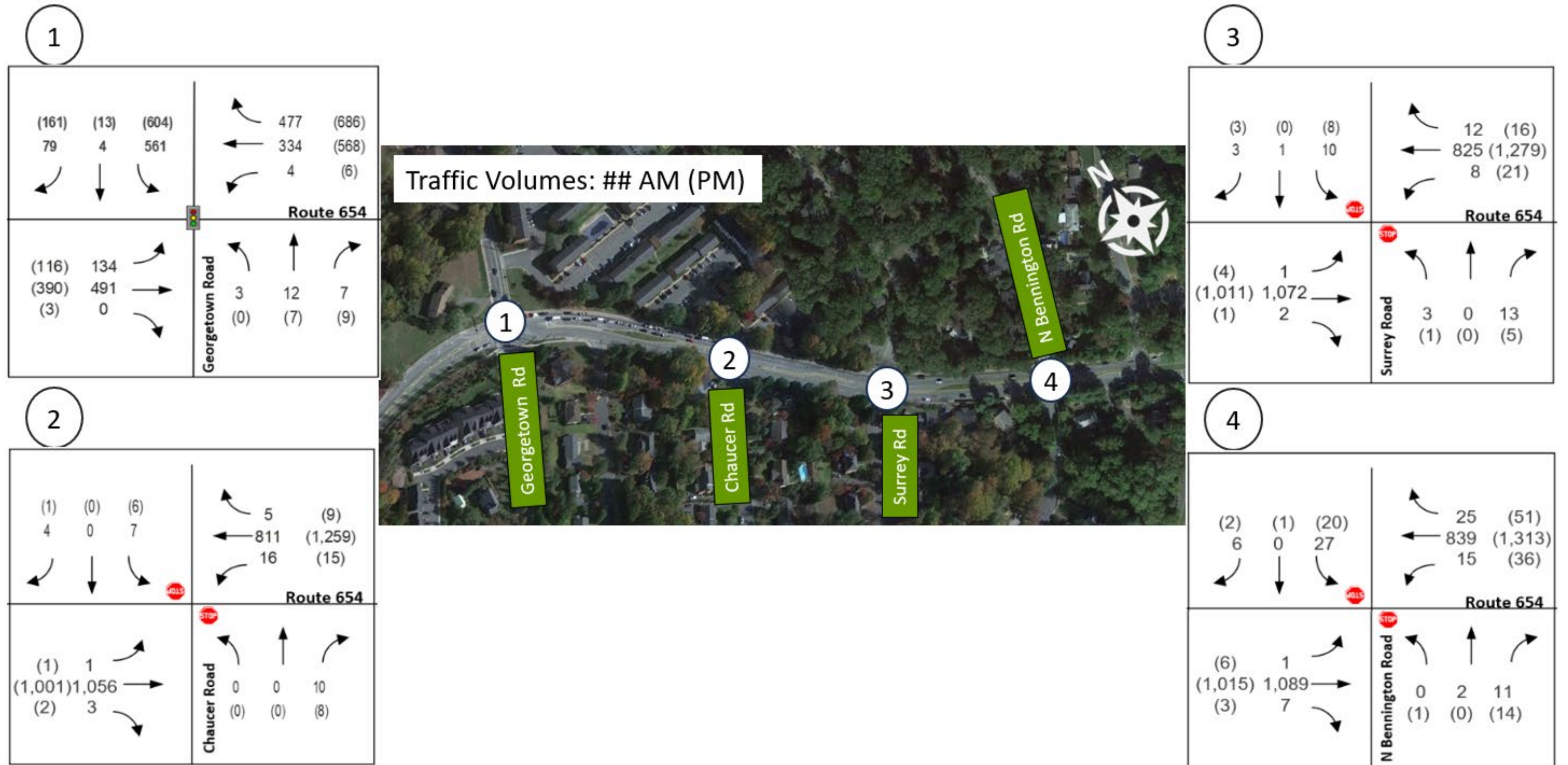
Figure 1-20. Barracks Road (Route 654) – 2035 Balanced Peak Hour Volumes (1 of 3)
