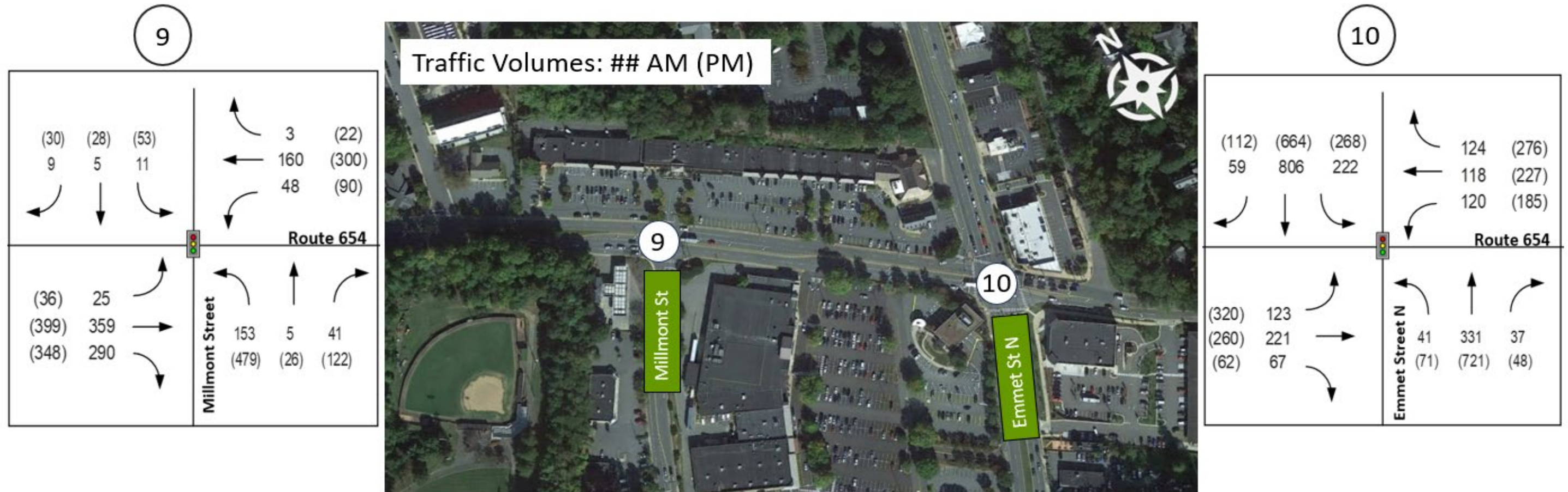
Figure 1-15. Barracks Road (Route 654) – Existing Conditions Peak Hour Volumes (3 of 3)
