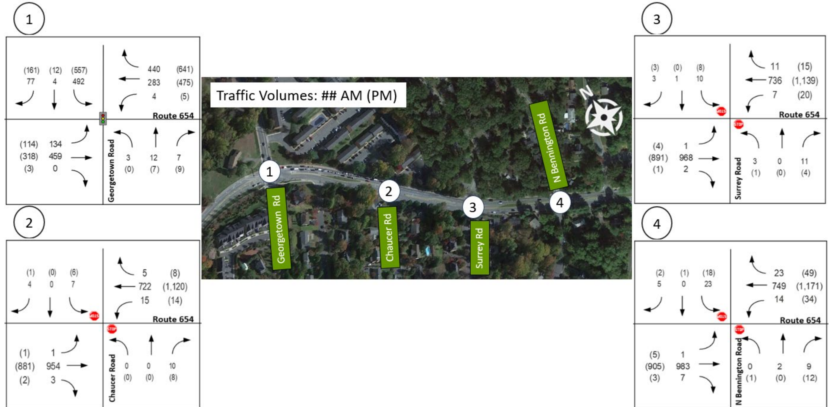
Figure 1-13. Barracks Road (Route 654) – Existing Conditions Peak Hour Volumes (1 of 3)
