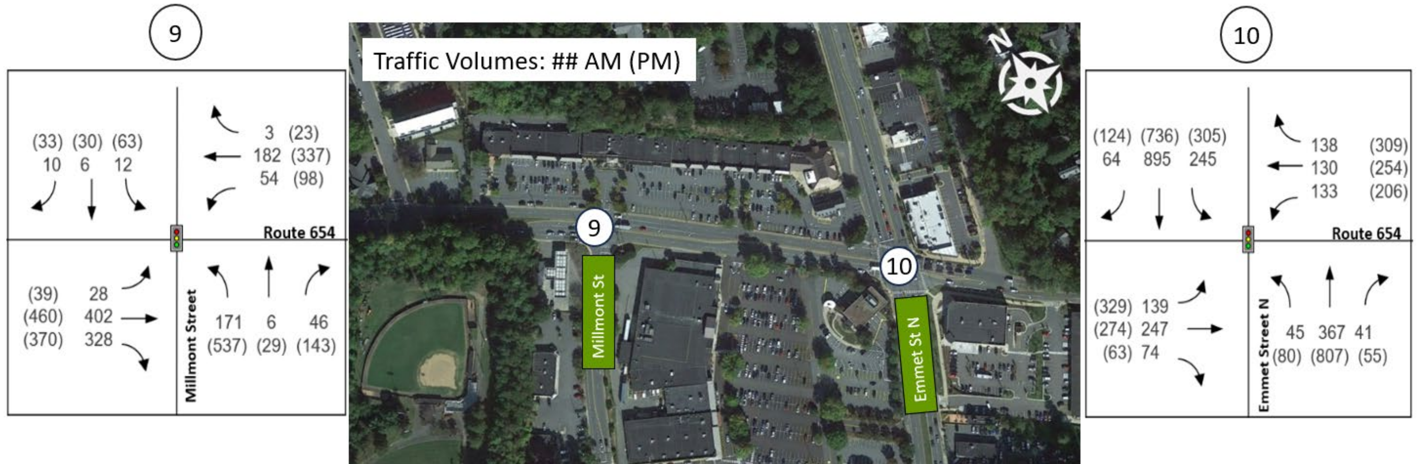
Figure 1-25. Barracks Road (Route 654) – 2045 Balanced Peak Hour Volumes (3 of 3)
