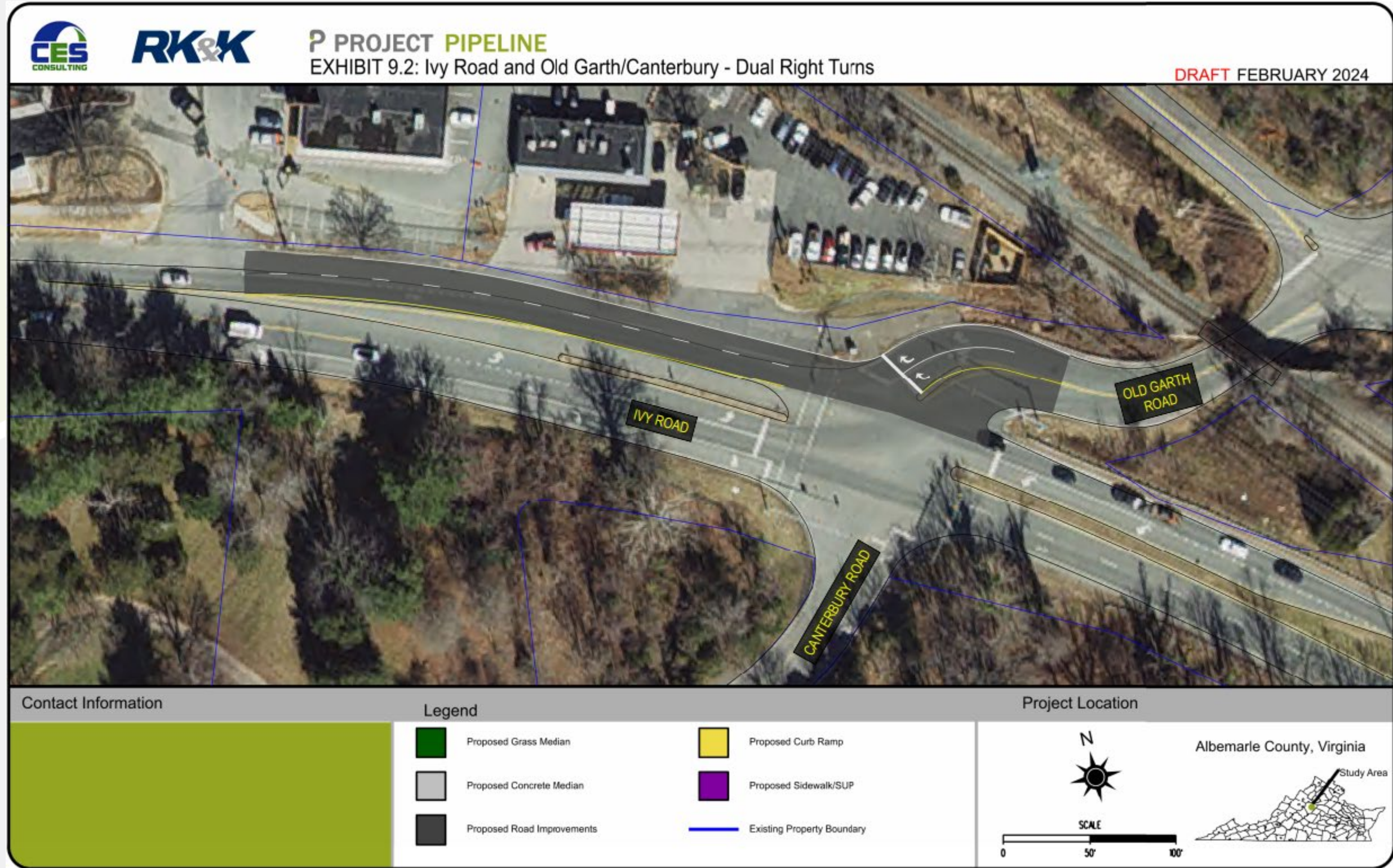
Figure 2-7 Ivy Road – Layout for Old Garth Road – Dual Right Turn
