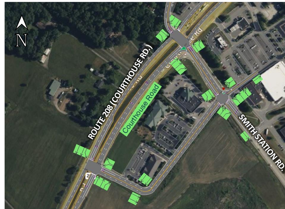
Figure 39: Smith Station Road Alternative 5a - Full Quadrant Roadway
