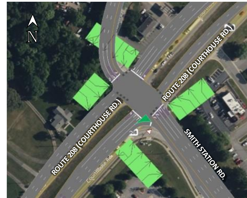
Figure 38: Smith Station Road Alternative 4 - Dual Northbound Left-Turn Lanes with Exclusive Southbound Lanes & Additional Westbound Through
