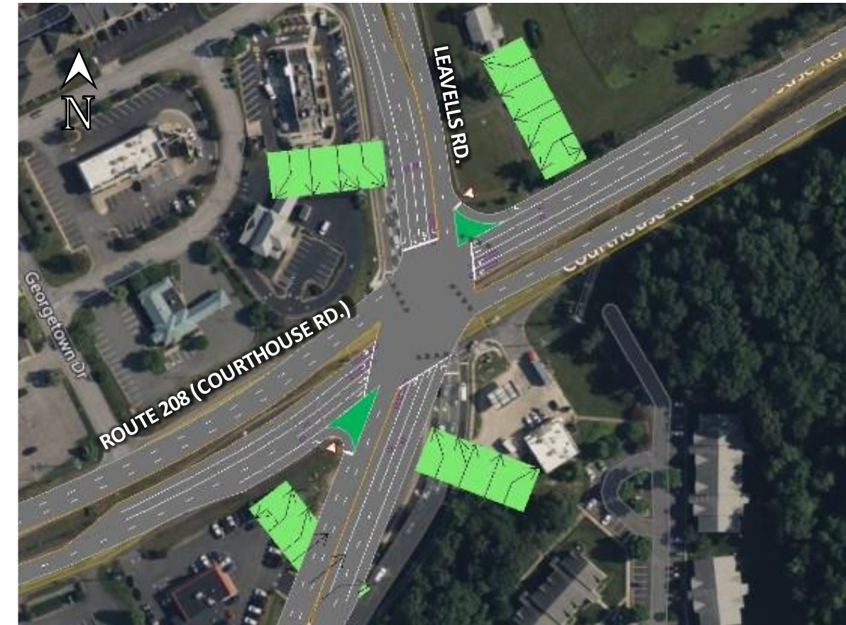
Figure 42: Leavells Road Alternative 2 - Dual Westbound Left-Turn Lanes
