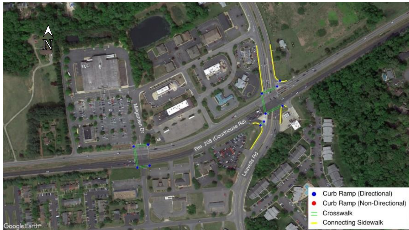
Figure 9: Existing Pedestrian Accommodations at Rte. 208 at Leavells Rd. and Millgarden Dr.
