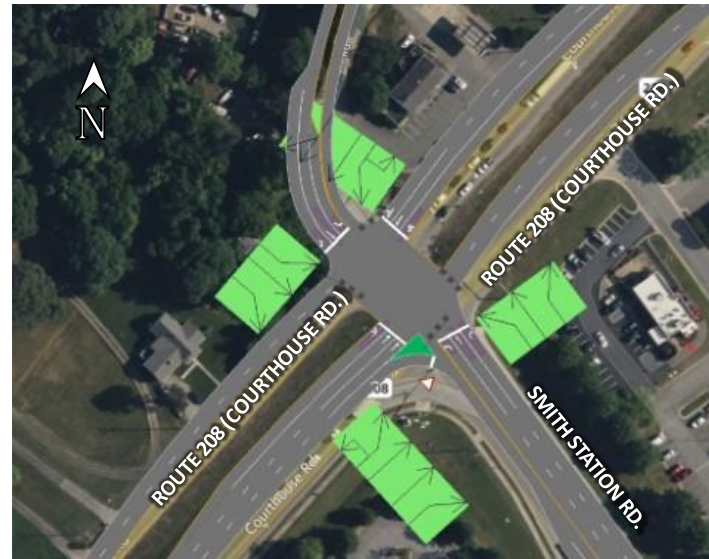
Figure 36: Smith Station Road Alternative 2 - Exclusive Southbound Lanes
