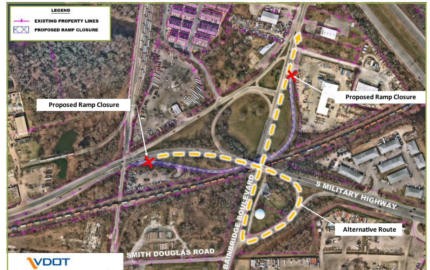
Figure 30: Phase 2 Concept - Eastbound S Military Highway to Northbound Bainbridge Boulevard Ramp Closure
