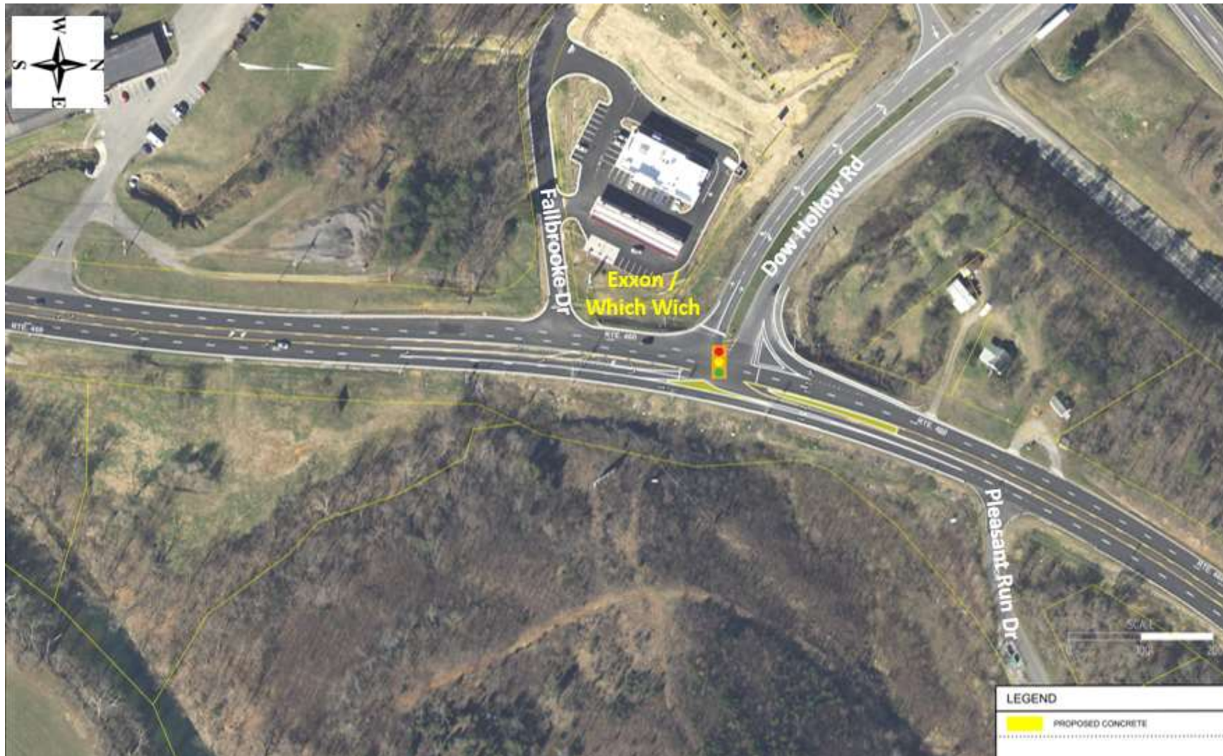
Figure 18: Route 11/460 at Dow Hollow Road Continuous Green-T
