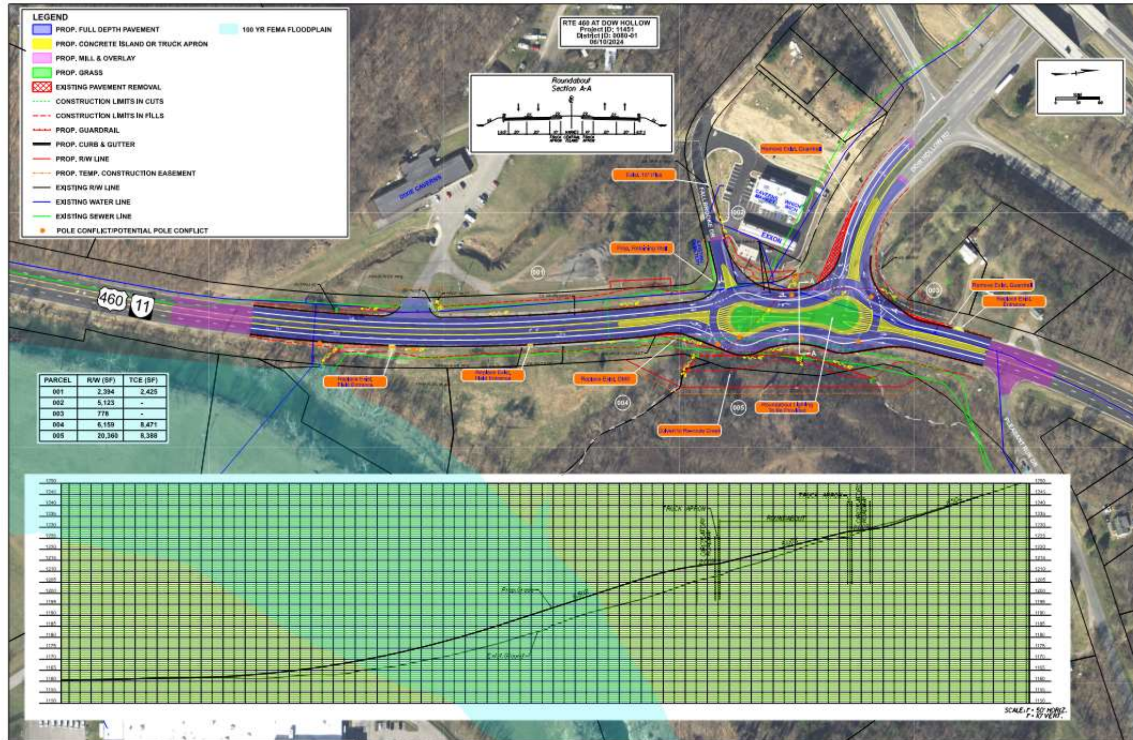
Figure 21: Route 11/460 at Dow Hollow Road Peanut Roundabout Preferred Alternative
