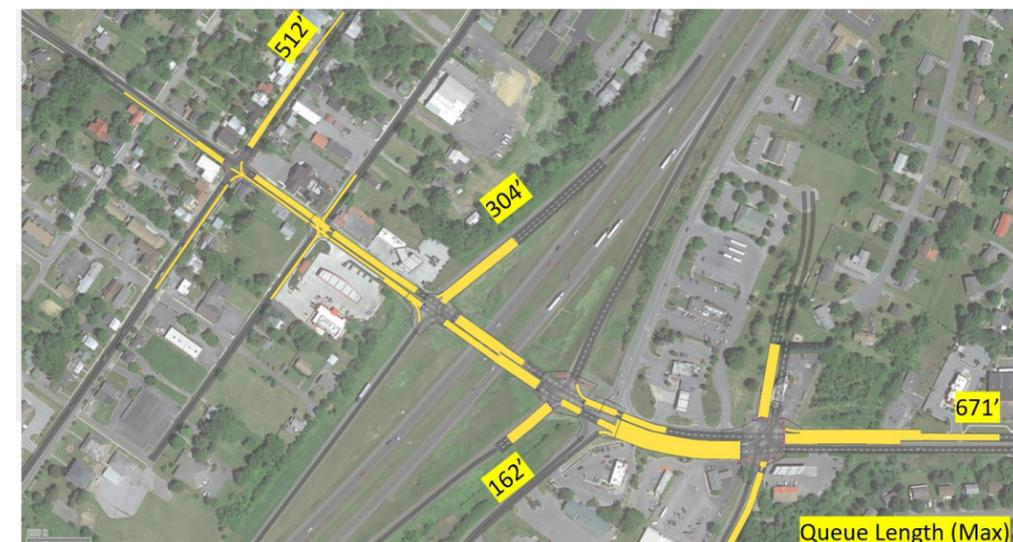
Figure 26. Alt.3B 2054 PM Peak Hour Maximum queue lengths
