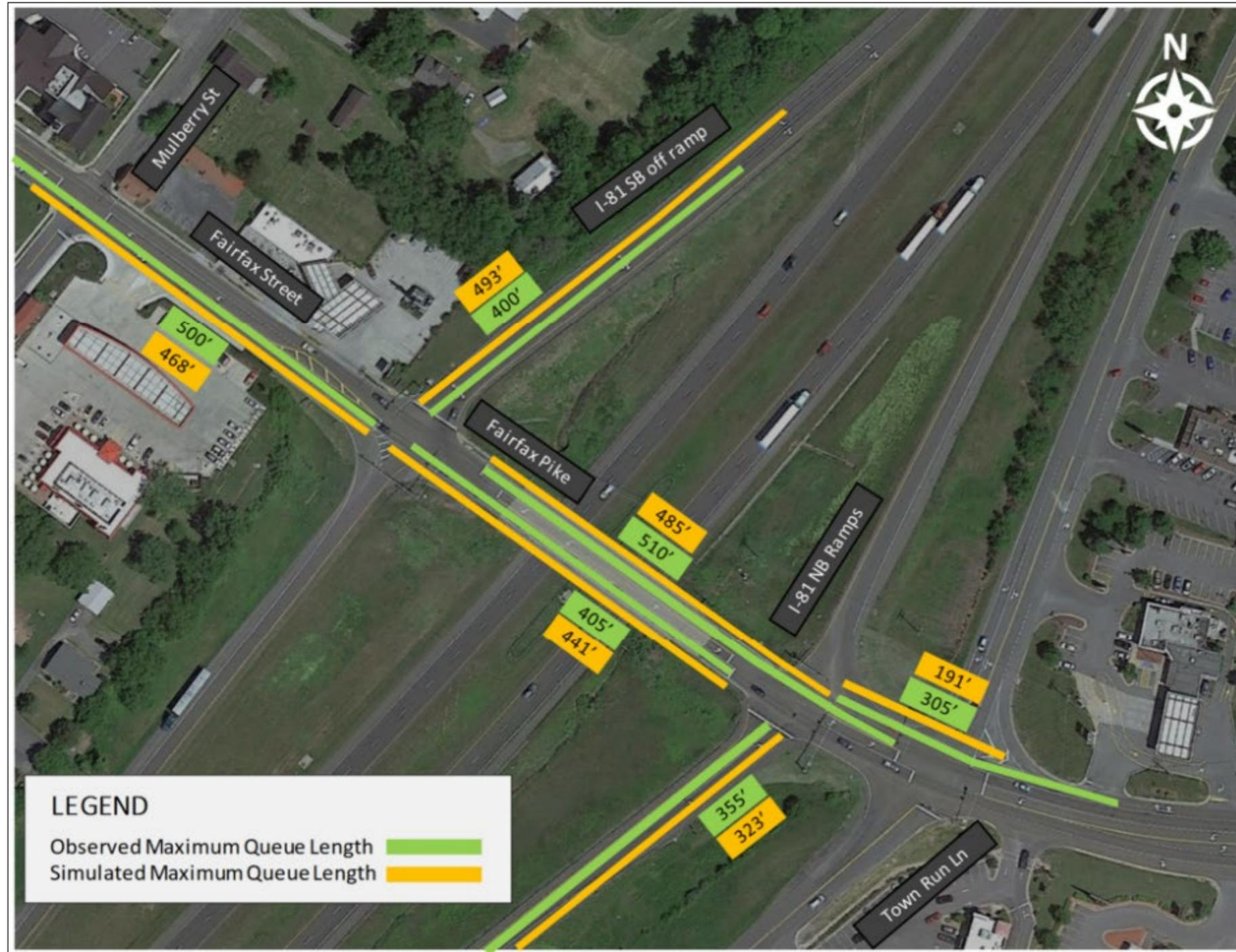
Figure 16. Observed vs. Simulated Queue Length Comparison in the PM Peak Hour
